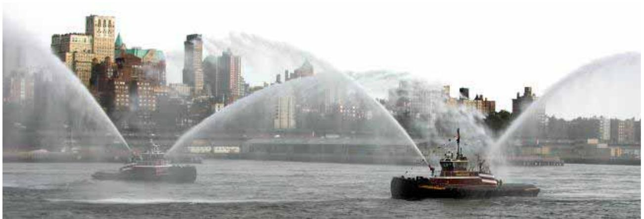
Engineering Manager Martin Costa says these tugs were built with “a shorter length to allow greater maneuverability in close quarter shipdocking operations.” Brian McAllister, in assisting on the design of these tugs, says, “These tugs are ideal in ports where efficiency is required.” The REID is currently in
