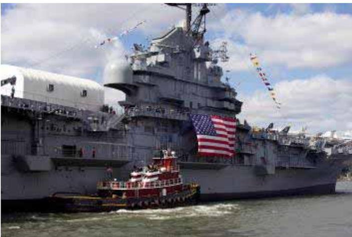
While the flotilla was underway in Upper New York Bay and the Hudson River, the main tow tug pulling on INTREPID'S bow was the 4,300 hp twin-screw ROWAN. The 6,000 hp tractor tug ROSEMARY was the tail tug, keeping the ship's stern from being blown cockeyed by the stiff wind. The 4,000 hp twin screw SISTERS was made up along the starboard hip with head, strap and stern lines, allowing the tug to offer forward or aft propulsion.
