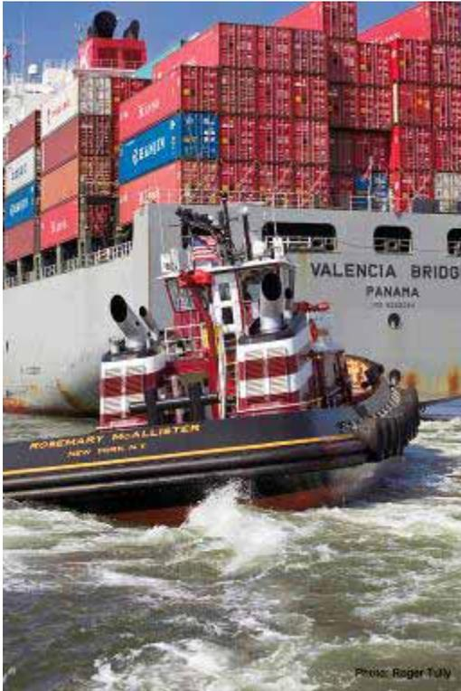
to pump more than 11,600 gallons of water or foam per minute. They have a certified bollard pull rating of 83 short tons and are equipped with JonRie escort winches. The tugs were designed by Jensen Maritime Consultants in Seattle and built by Eastern Shipbuilding, Inc. in Panama City, FL.
